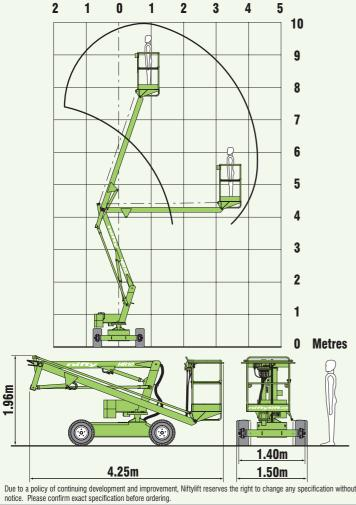
With a super narrow version at only 1.40m wide, operators can work even in the tightest working environments.
